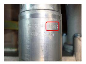
The date of production of the steel wire mesh hoses has to be documented during the commissioning. For engines which are already in operation, the date of production must be checked and documented within the next regular service operation.
